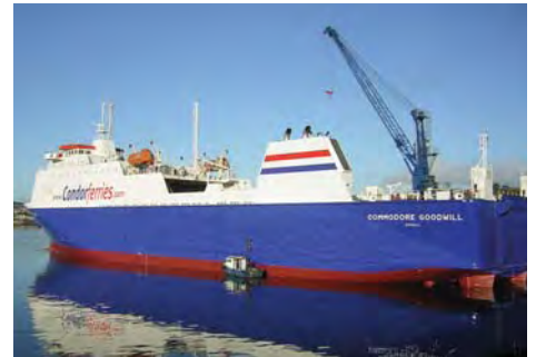
Interthane®990 applied over Intergard®263 on topsides and superstructure
