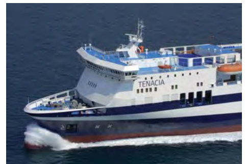
Interthane®990 applied to topside and decks
